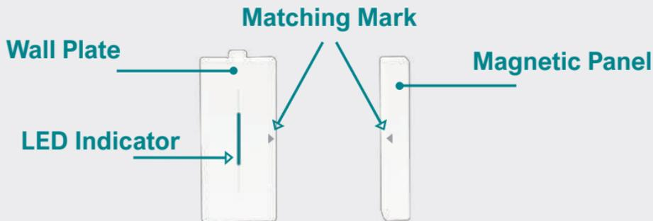
It consists of two parts: transmitter (main panel) and magnetic panel, when the transmitter and magnetic panel are separated to a certain distance, the transmitter sends out an alarm.
